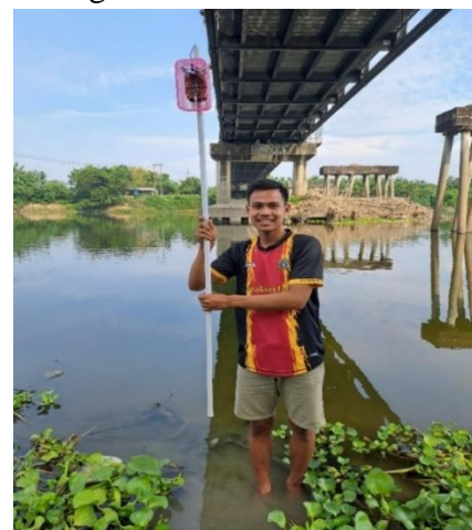
Figure 12. Deployment of water level system in Bengawan Solo
